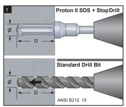
Drill hole into the base material to the depth of embedment required, using a Proton SDS + Stop Drill, or a standard drill bit.
